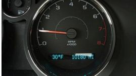
In addition, these thermometers can also read lower if rain water hits the sensors and evaporates while the car is at a higher speed. Overall, car thermometers give relatively accurate readings, but for various reasons they can be incorrect, so they should not be used as the absolute authority, Strait said.
